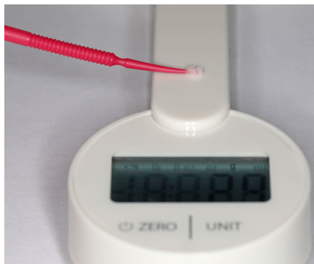
FIGURE 14 A disposable applicator with a constriction at the end of the handle is shown here with very slight bending of the tip when an application force of 29 grams is applied.
