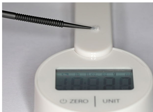
FIGURE 15 This disposable applicator without a constriction is applying a force of 27 grams with no bending of the tip.
