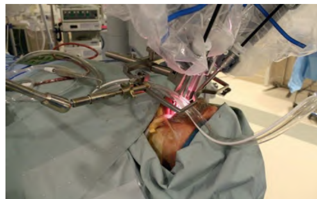
Figure 7-21 The da Vinci surgical robot (Intuitive, Sunnyvale, CA, USA) is docked and all three arms (endoscope, monopolar cautery, and Maryland forceps) are advanced into the oral cavity.
