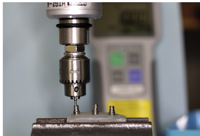
Figure 2. Tightening abutment screws with digital torque measuring device.
